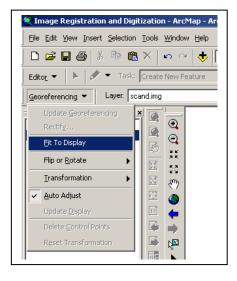
In the Georeferencing drop down box select the Fit to Display
