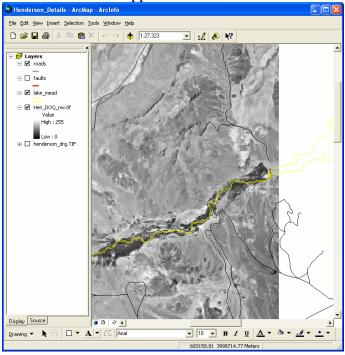
Notice the how the water goes thru the wash. It doesn't fill the whole wash. Notice also the darker tones are vegetation in and along the wash.
