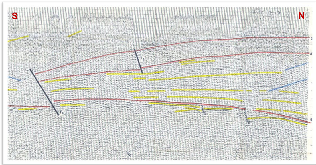
Seismic line ZU2 running north-south, located east of the Ribera Alta diapir. Vertical axis in time.
